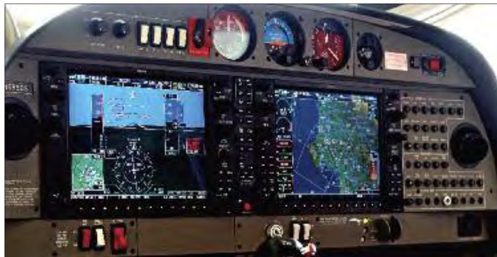
The cabin of the DA40 XLS features a sports car-like interior with a center-stick design (left) that appears to grow out of the seats (top). The aircraft is equipped with Garmin's G1000 glass panel (middle), and Synthetic Vision Technology offers a 3-D view of surrounding terrain and potential obstacles.
